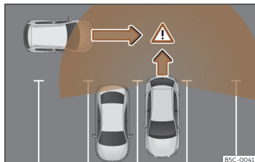
Fig. 163 Diagram of the parking assistant: detected area around the vehicle that is driving off.
