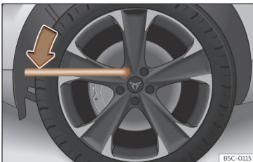
Fig. 243 Tyre change: slacken the wheel bolts.
