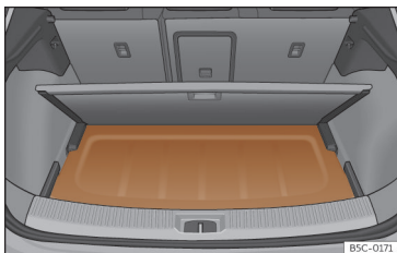
Fig. 182 In the boot: fitting the rear shelf.
