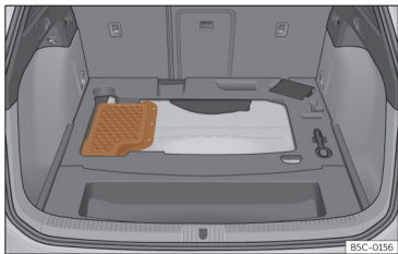
Fig. 233 Hybrid vehicles (PHEV): location of the battery in the luggage compartment
