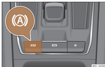
Fig. 154 In the lower part of the centre console: Auto Hold function button.
