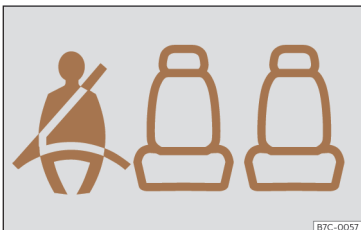
Fig. 19 Instrument cluster: indication of the status of the rear seat seat belts.
