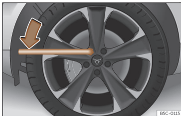
Fig. 236 Tyre change: slacken the wheel bolts.
