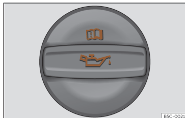
Fig. 226 Oil filler cap cover in the engine compartment.
