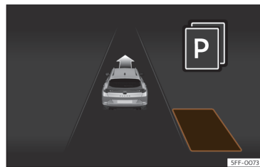
Fig. 158 On the instrument panel display: display of the assisted parking system with decreased visibility.
