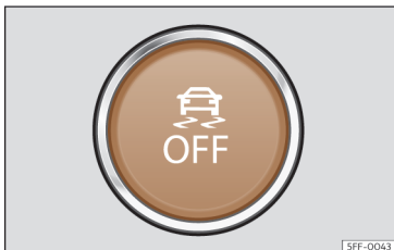
Fig. 124 On the lower part of the centre console: ESC on/off button
