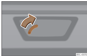
Fig. 84 Luggage compartment: manual release.
