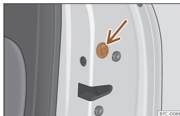
Fig. 77 Locking the door manually.
