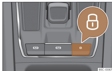
Fig. 75 On the centre console: central locking button
