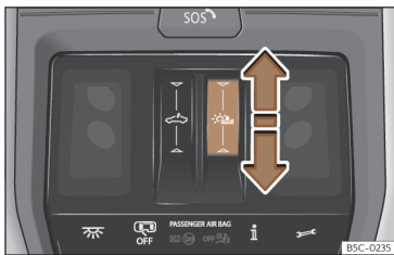
Fig. 88 On the headliner: operate the sun blind.
