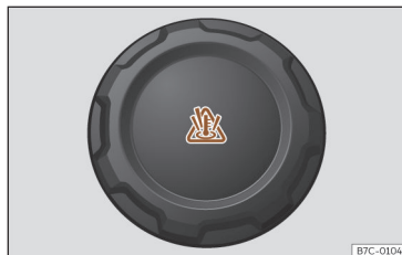
Fig. 220 Front compartment: coolant expansion tank cap.
