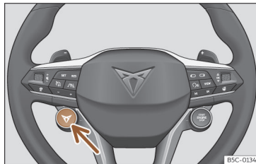
Fig. 123 Multifunction steering wheel: button to change the driving profile.
