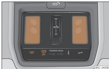
Fig. 106 Detail of headliner: front interior lighting.
