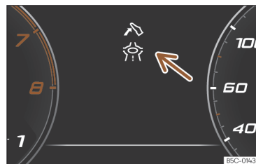
Fig. 135 Eco-efficient driving assistance indication (schematic representation).
