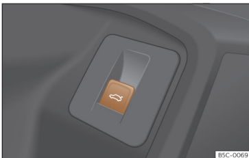
Fig. 81 On the driver's door: button for opening and closing the rear lid.
