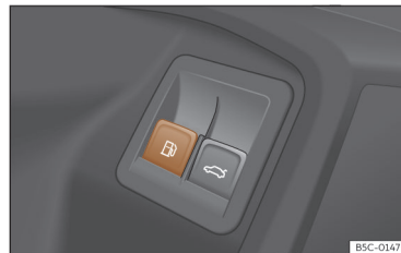
Fig. 202 Driver's door: tank cover release.
