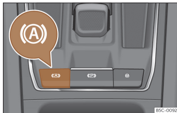
Fig. 155 In the lower part of the centre console: Auto Hold function button.
