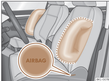
Fig. 32 Driver's seat and passenger seat side airbags.
