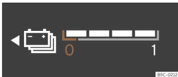
Fig. 5 Digital instrument cluster: battery level indicator.
