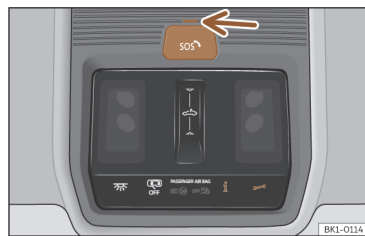
Fig. 51 On the roof console: controls for voice services.
