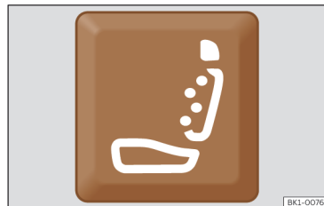
Fig. 86 On the lateral underside of the driver and passenger seats: massage function button.
