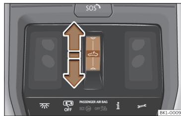
Fig. 96 On the interior roof lining: function button to operate the sun blind.
