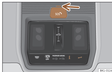
Fig. 45 On the roof console: controls for voice services.
