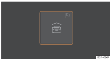
Fig. 135 Infotainment system: parking space with guided route for the navigation system (depending on country and vehicle equipment).
